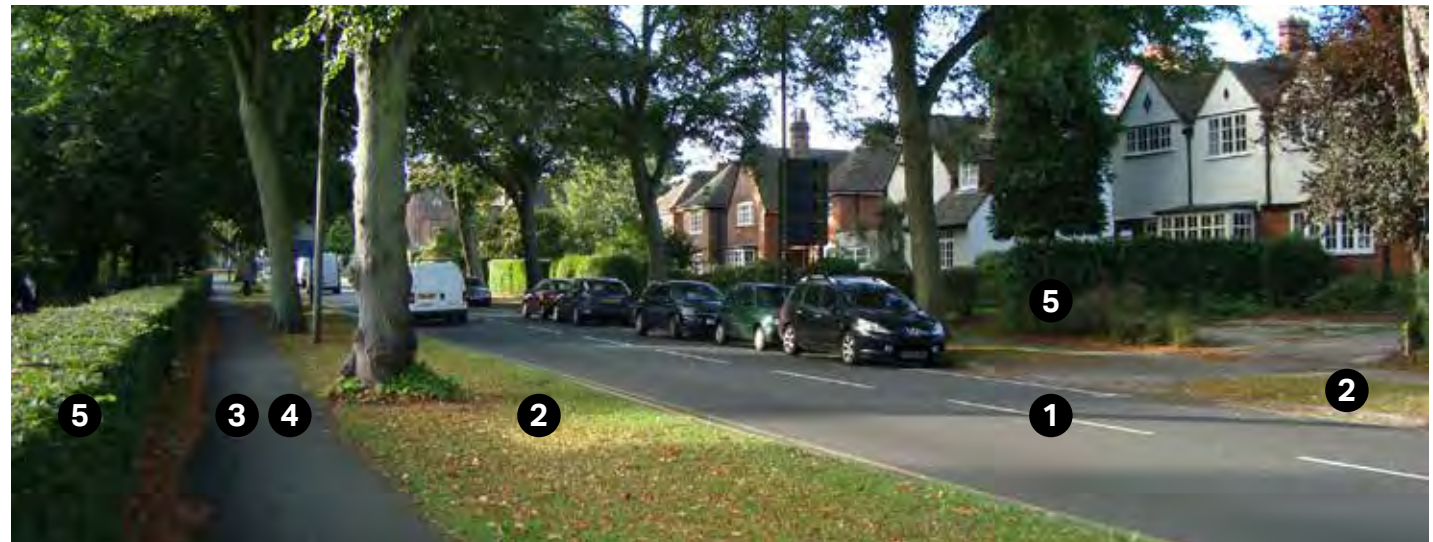
Figure 74: An example showing primary road framed by wide tree verges in a residential neighbourhood. It is recommended that cycle provisions are separated from moving traffic and that parking bays, where required, are inset into the verges to avoid impeding the movement of pedestrians and vehicles.
