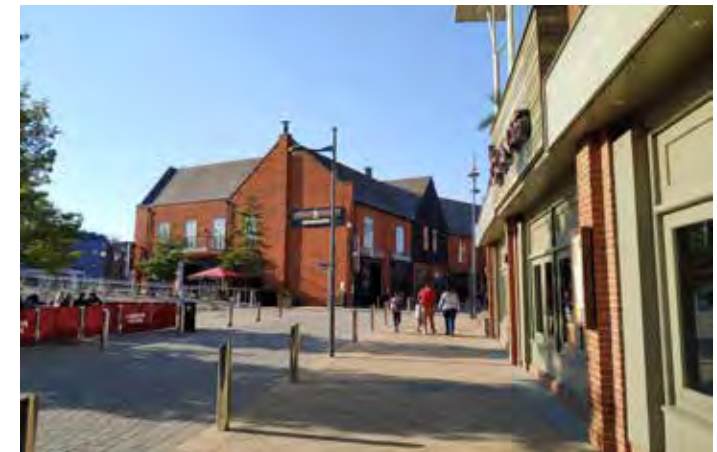
Figure 115: Example of lighting columns set at heights and positions to provide light to both pedestrian areas and the carriageway. It is recommended that LED lighting is used due to higher energy efficiency and power cost savings.
