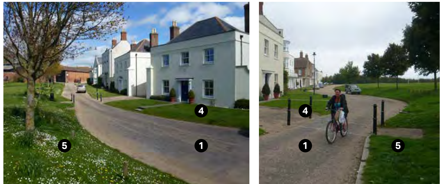
Figure 83: Examples of edge lanes, with low-speed roads shared between motor vehicles and cyclists, and opportunities for on-street parking (note: some localities may prefer clearly defined footways and parking bays).
