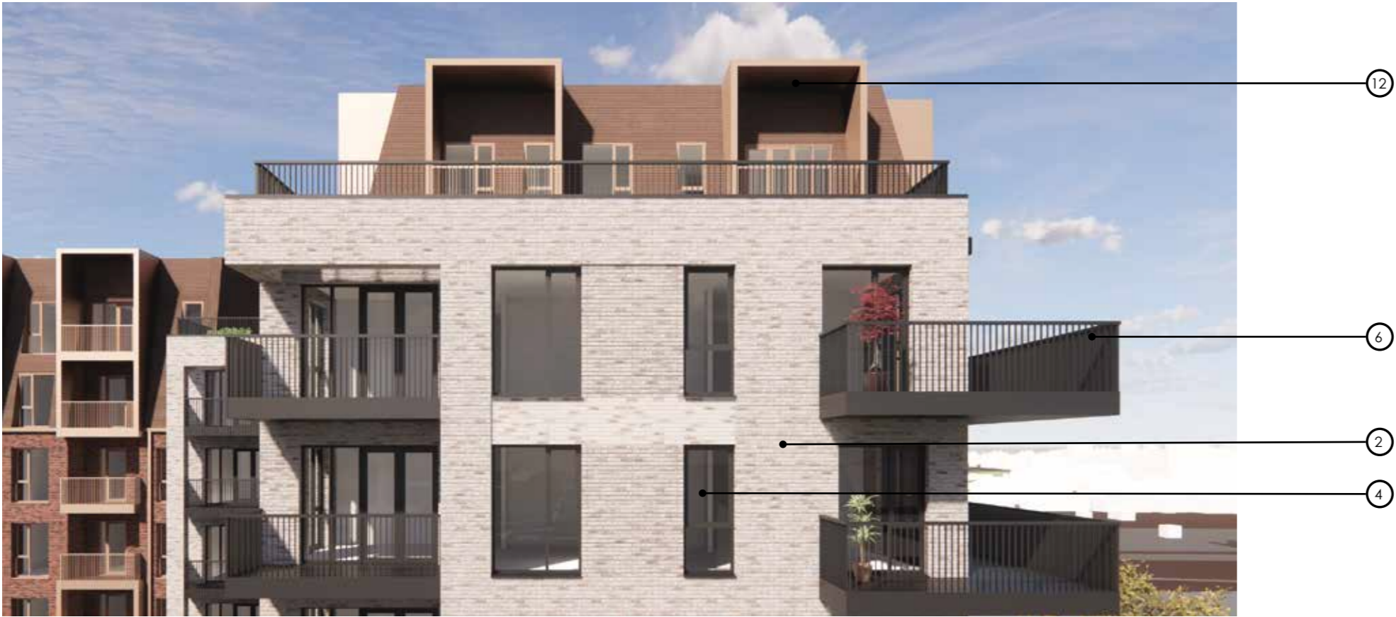
^ Both inset and cantilever balconies to create variation and for privacy
